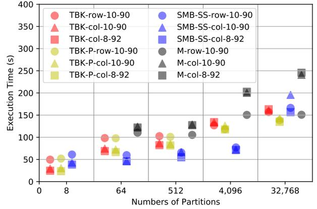
Figure 11: Partitioning 1 billion 100-byte tuples with skew using a single thread.
