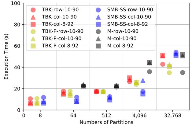
Figure 13: Partitioning 1 billion 100-byte tuples with skew using 4 threads.
