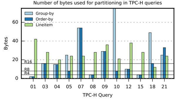
Figure 2: Width of tuple required for partitioning to execute various TPC-H queries. The lines at 4, 8, and 16 bytes indicates the tuple width considered by related work. For this analysis, we assume that the *Decimal*, *Date*, and *year* columns occupy 8, 8, and 4 bytes, respectively, while a variable-length attribute uses its maximal length.
