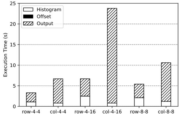
Figure 3: Storage format impact on Radix Partitioning 1 billion tuples with 32 partitions using just 1 thread. The dataset names are coded as *format-keysize-payloadsize*; for example, *col-4-16* is a dataset with two columns, 4 and 16 bytes, stored in a columnar storage format. The three key phases of radix partitioning are shown, the initial histogram creation phase, creating offsets, and the final output. The second phase takes negligible amount of time.
