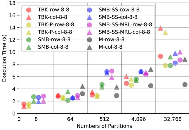
Figure 12: Partitioning 1 billion 16-byte (8-8) tuples with skew using 4 threads.
