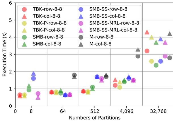
Figure 14: Partitioning 1 billion 16-byte (8-8) tuples with skew using 16 threads.
