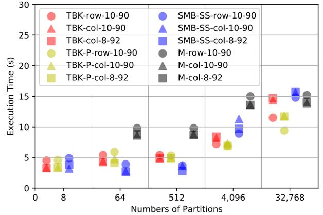
Figure 9: **Partitioning 1 billion 100-byte tuples using 16 threads.**
