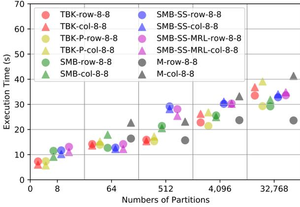
Figure 10: Partitioning 1 billion 16-byte tuples with skew using a single thread.
