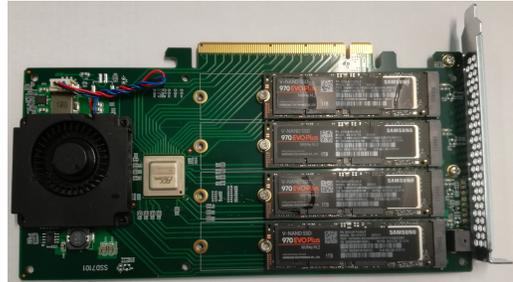
The controller hosts the four SSDs and is itself connected using 16 PCIe 3.0 lanes. It either simply exposes the SSDs to the operating system as separate devices or serves as a hardware RAID controller. We validated that in the former mode, which we use for most experiments, the controller does not add any overhead. Our system has an Intel Core i9-9900K CPU with 8 cores (16 hyper-threads) and 64 GB of RAM.
