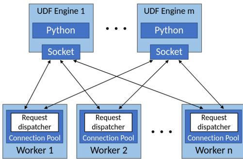
Figure 3: Overview over the UDF engine pool
